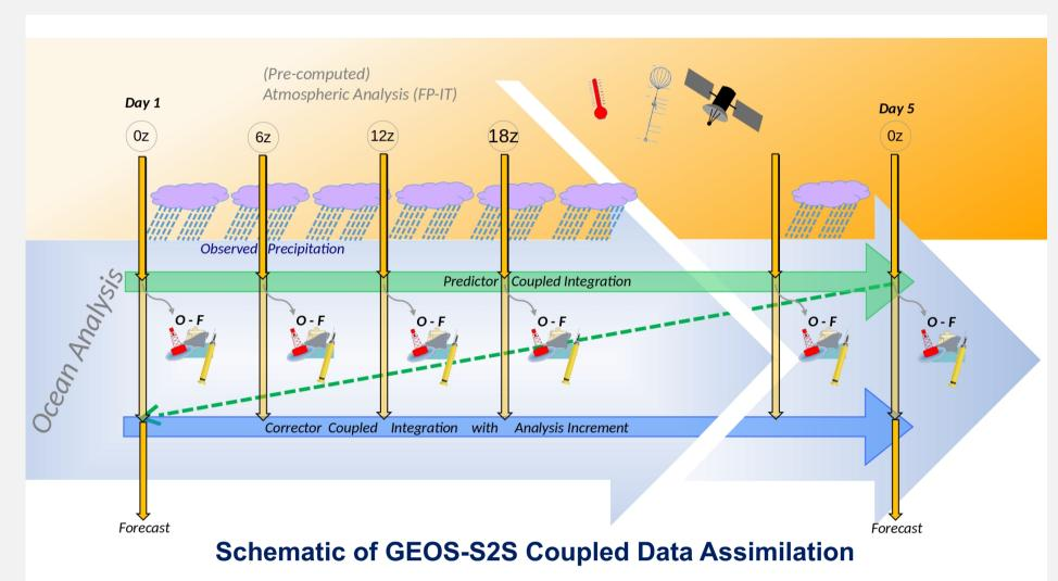
The GEOS-S2S AODAS includes an ocean predictor sequence (the green line near the middle of the figure) and a corrector sequence (the blue line along the bottom of the figure). As the predictor segment proceeds, every 6-hours the "ocean observers" are used to compute the departure of the model trajectory. These innovations are then used to perform an LETKF analysis. The analysis increments are applied over the first 18 hours of the corrector sequence.
