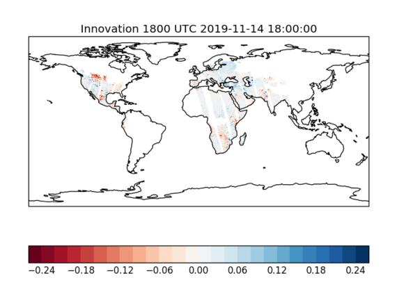
ASCAT SW is interpolated to the model grid using an inverse distance weighting scheme.
