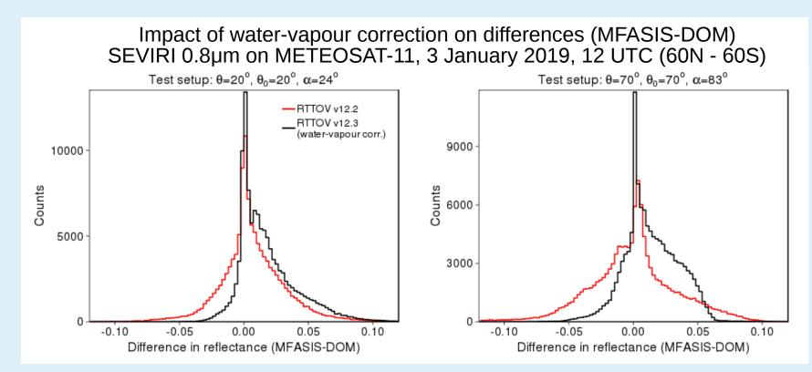
→ Errors in SEVIRI 0.8µm channel successfully reduced to same magnitude as other channels
