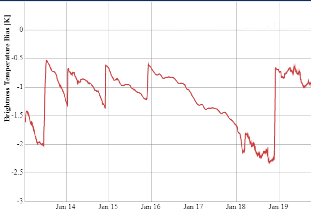
Time Series of Bias in Meteosat-10/SEVIRI IR13.4 channel from GSICS Re-Analysis Correction for standard scene (267K) based on inter-calibration with Metop-B/IASI. From GSICS Plotting Tool: gsics.tools.eumetsat.int/plotter
