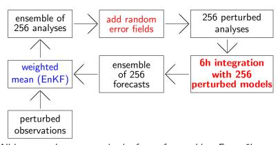
All inputs and output are in the form of ensembles. Every 6h, the new observations are perturbed randomly. Isotropic random fields are added to the analyses and different configurations of the model physics are used.
