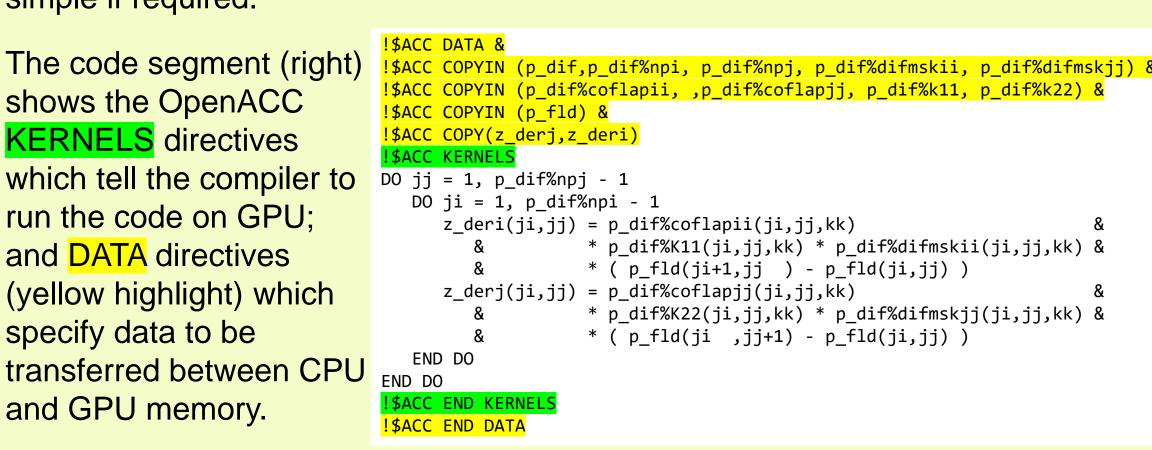
This is an explicit memory management approach which is flexible and powerful, but depends on the developer to ensure correct transfers of data between system and GPU memory. Memory management is often the bigger part of the task, and if incomplete will lead to runtime errors or incorrect results.
