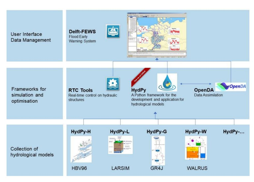
HydPy as a unifying interface for the seamless integration of multiple hydrological models in forecasting workflows.
