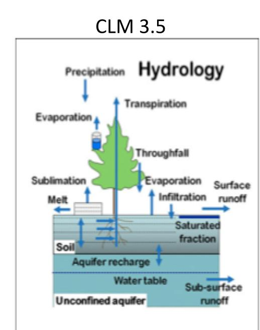
CLM3.5 simulates movement of moisture between 10 soil layers is calculated using Richard's equation. The bottom soil layer is also coupled with an unconfined aquifer to account for groundwater recharge and discharge processes. There is no representation of the confined aquifer in the model.
