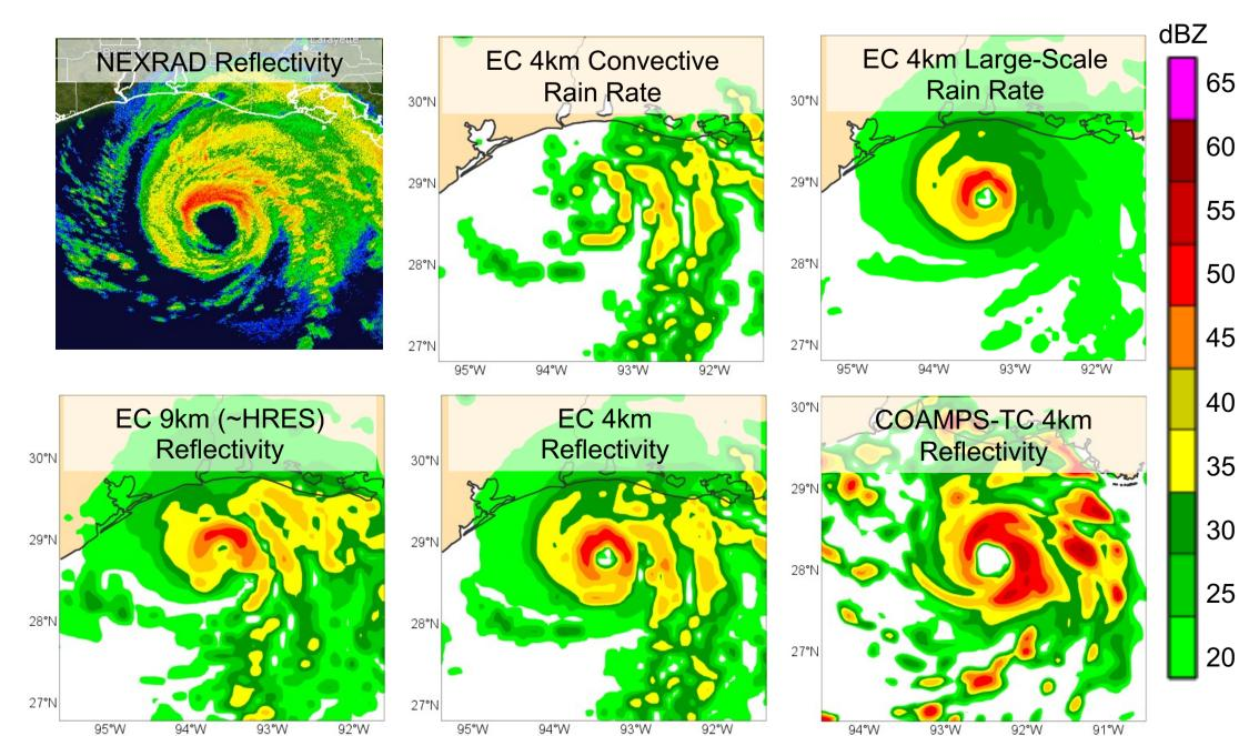
Using simulated radar reflectivity and forecast rain rates to investigate TC structure and intensity at different model resolutions<sup>3,4</sup>
