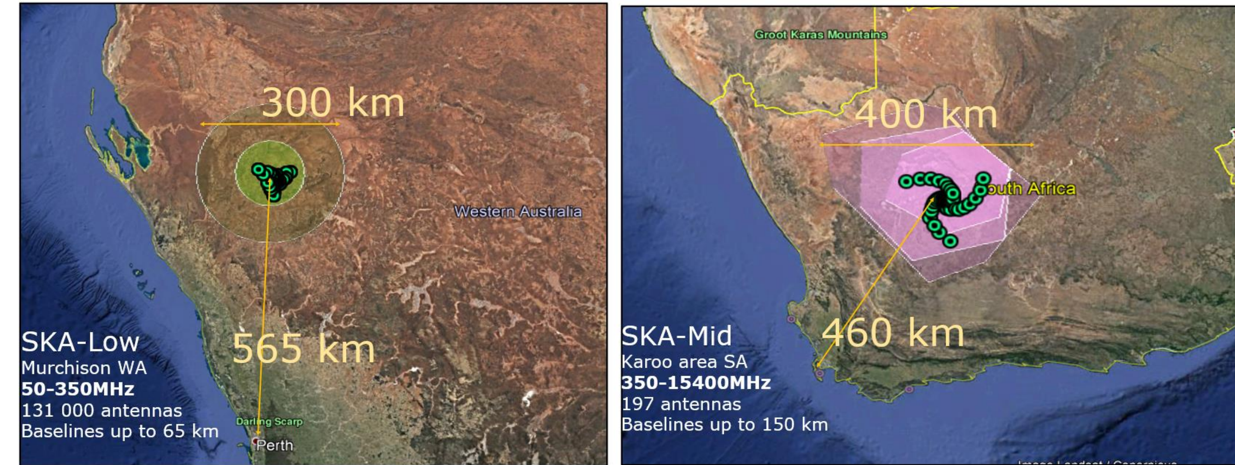
SKA-Low and SKA-Mid sites with their respective RQZs and antenna configurations
