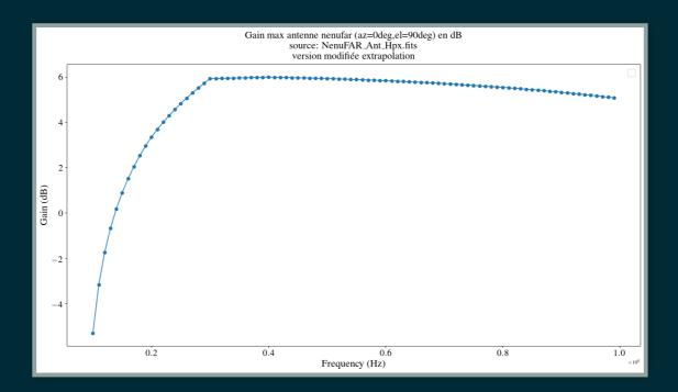
Antenna max gain vs. frequency as simulated with NEC2
