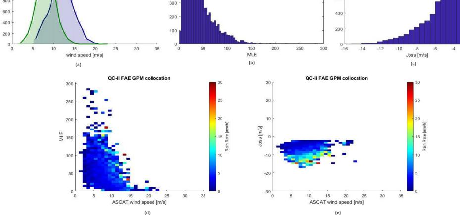
winds remain of acceptable quality. The winds distorted by rain (clouds) are clearly the segregated FAE, by resulting in deformed а speed distribution, as well as much elevated MLE and Joss, that all can be potentially related to WVC rain rate.
