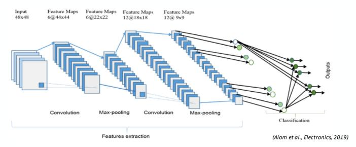
The overall architecture of the Convolutional Neural Network (ConvNet) includes an input layer, multiple alternating convolution and max-pooling layers, one fully-connected layer and one classification layer.
