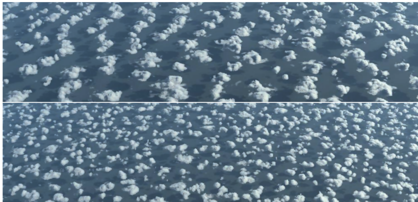
Figure 1. Virtual photograph of LES simulations at a cruising altitude of 15 km. Top panel: cloud formation of a simulation driven by 3D radiation (TenStream with sun in the east, i.e. right ( \varphi = 90^\circ )). Lower-panel: cloud formation of a simulation which was performed with 1D radiation (Two-stream). The specific model setup is the same as referenced in fig. 2 i.e., no background wind and a continental land surface. The simulations differ with respect to cloud size distributions and the organization in cloud streets, the cloud fraction though is the same (27%). The visualization was performed with a physically correct rendering with MYSTIC (MonteCarlo solver in libRadtran (Mayer, 2009, Emde et al. 2015)). SZA = 60°
