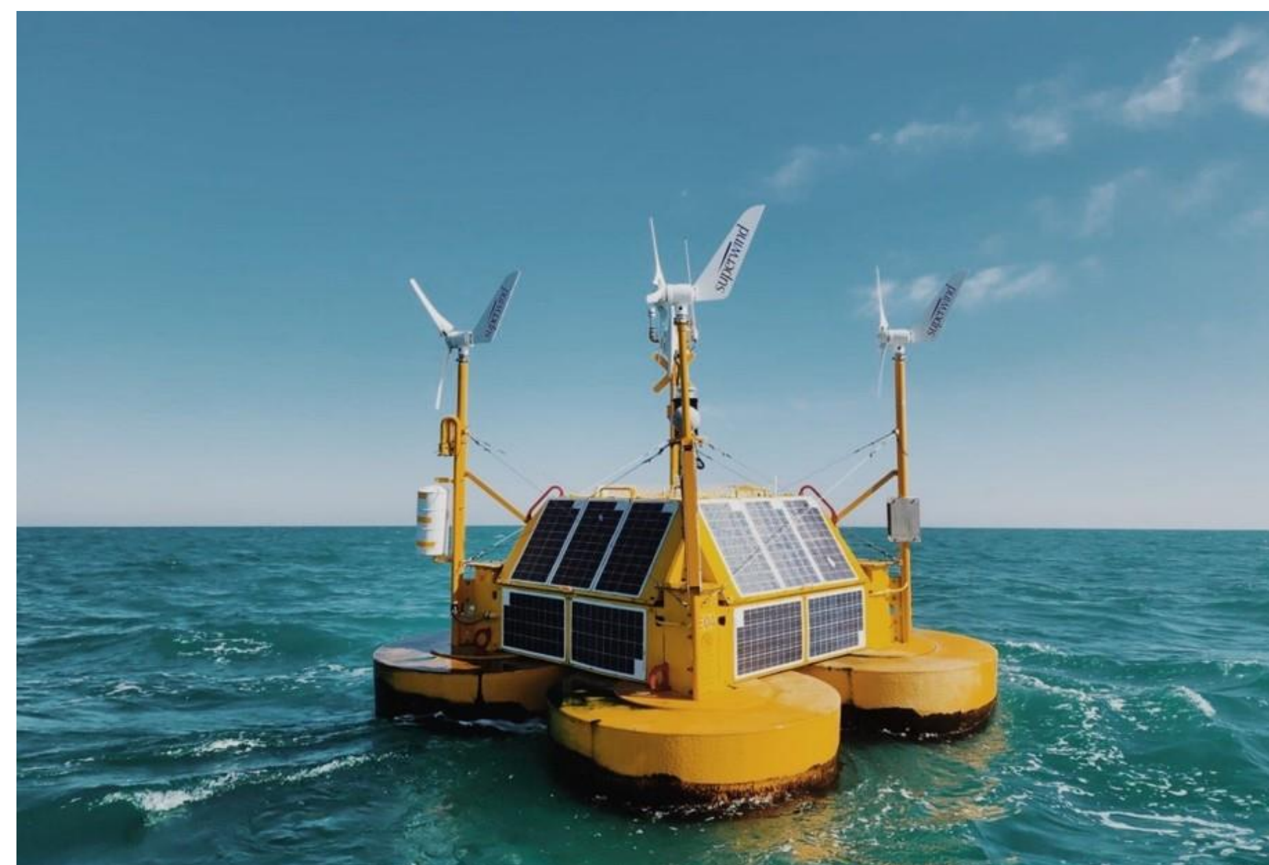
Figure 1. EOLOS FLS200 buoy. Wave sensor is mounted on buoy.
