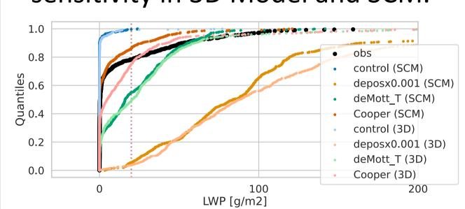
Setup test: LWP quantiles for sensitivity tests in 3D model and SCM for December 2019
