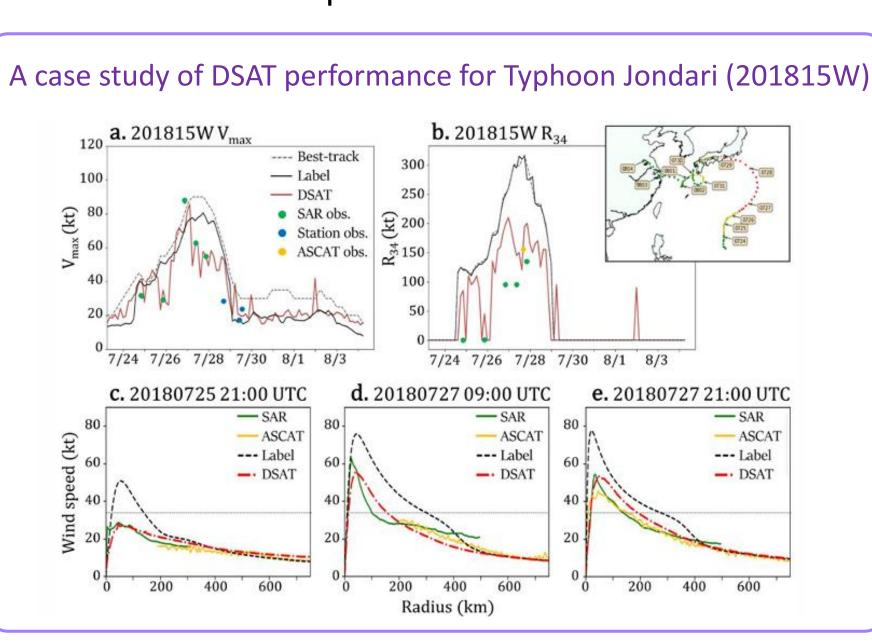
The DSAT model has comparable accuracy for intensity ( $V_{max}$ ) estimates compared with **SATCON** and better accuracy for size  $(R_{34})$  estimates compared with MTCSWA for global TCs during 2017–2018.
