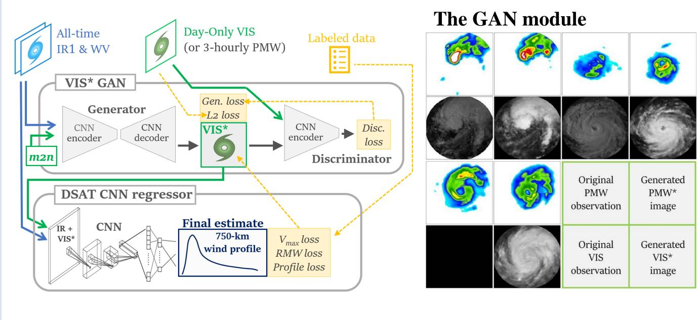
The hybrid GAN-CNN DSAT model includes a GAN module for generating mimic VIS\* images based on the input IR and WV images, and a DSAT polar-CNN regressor that uses IR and VIS\* images to estimate TC wind profiles within 750 km of the TC center.
