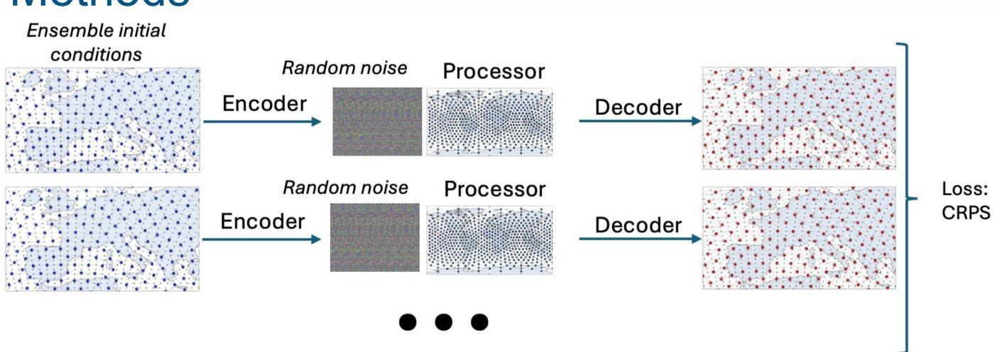
We use the AIFS-CRPS architecture [1] that creates ensemble members by conditioning the processor on randomly sampled noise in each step. The loss over the members is computed by the almost fair CRPS:
