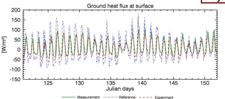
Ground heat flux substantially overestimated by TERRA, with the skin temperature formulation it is significantly reduced and much closer to the measurements
