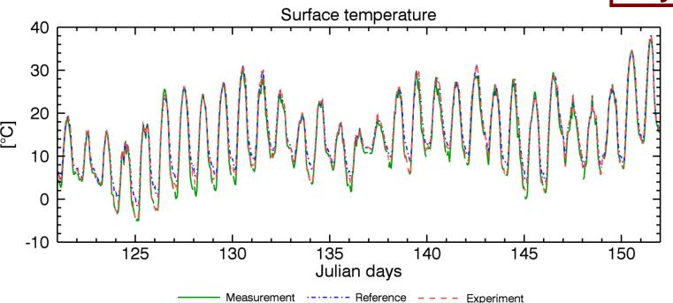
Amplitude of the diurnal cycle of the surface temperature in TERRA systematically underestimated (clear nocturnal warm bias), with the skin temperature formulation it is substantially increased and much closer to the measurements
