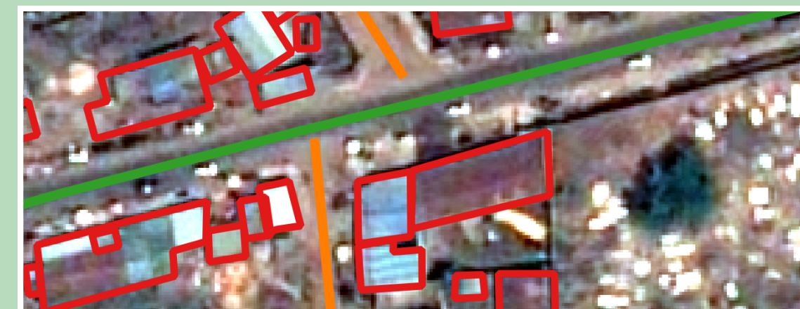
Fig 2. Model labeling, red for buildings, green for paved roads and orange for unpaved roads
