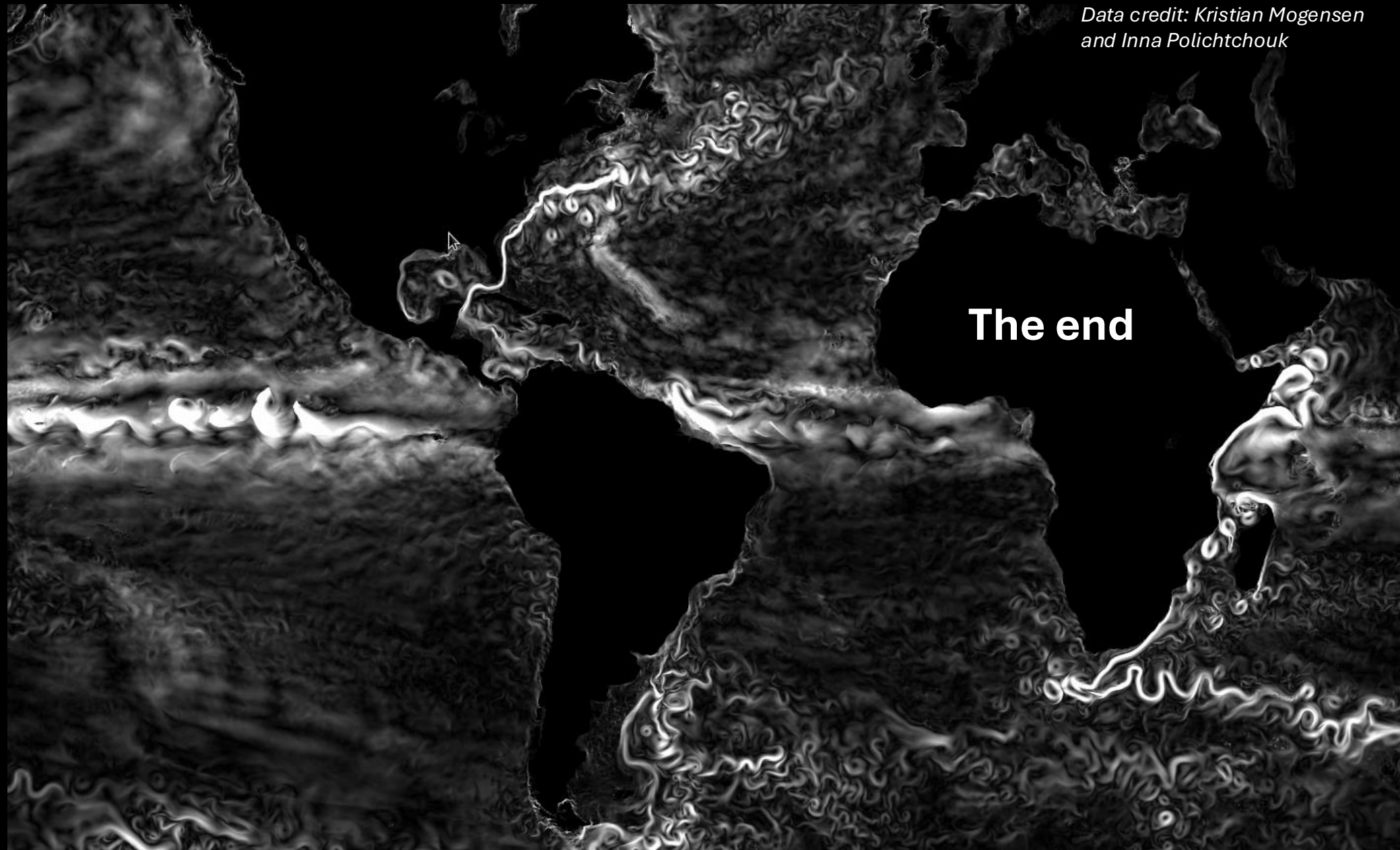
Snapshot of surface current speeds in the ECMWF global coupled model (IFS ~4 km, NEMO ~8 km)
